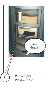
The **secondary draft control** lever regulates the amount of air that is needed to reburn exhaust gases that are produced in the fireplace during the wood burning process. A portion of this secondary air circulates from the top to the door and helps to keep the glass window clean.
